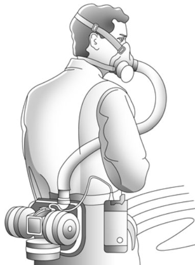
Tight-Fitting Half Facepiece Powered Air-Purifying Respirator (PAPR) APF=50 Needs to be fit tested
