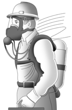
Self-Contained Breathing Apparatus (SCBA) Atmosphere-supplying, or Supplied-air respirator (SAR), which provides clean air from an uncontaminated source Needs to be fit tested APF=10,000
